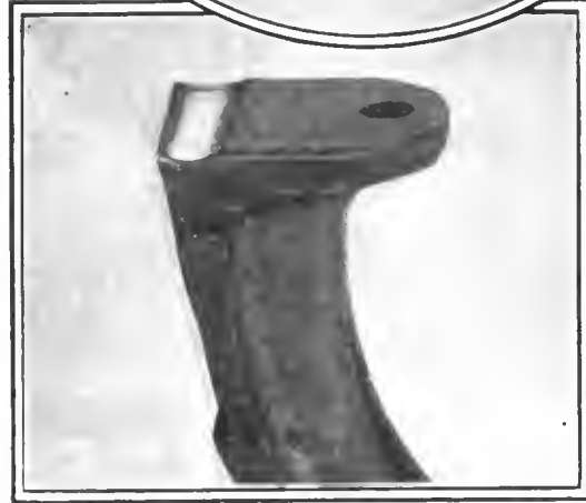
Fig. 2—Showing a worn brakeshoe after having been repaired by the oxy-acetylene process
